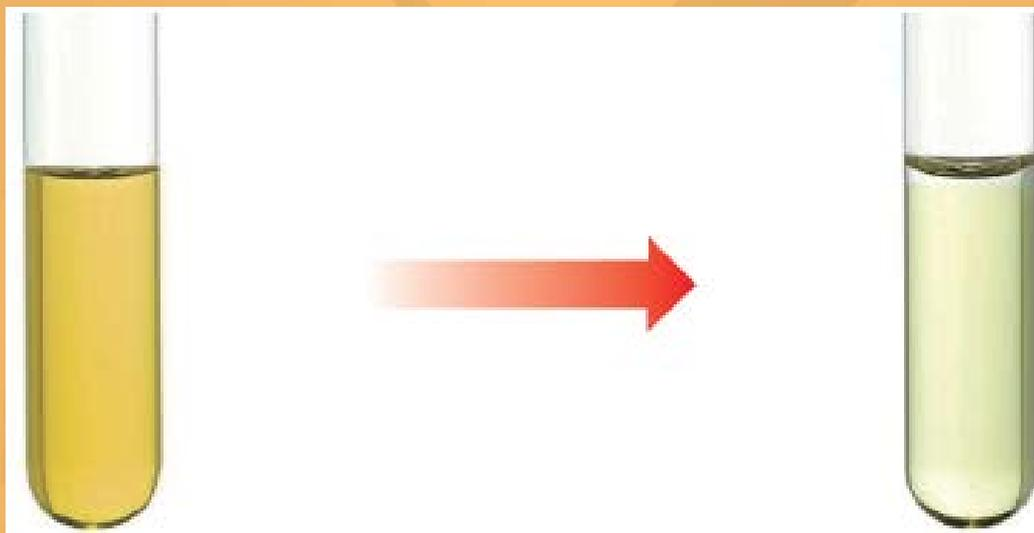
**Fe<sup>3+</sup>(aq) ions (left) are reduced to Fe<sup>2+</sup>(aq) ions (right) during a redox reaction**
