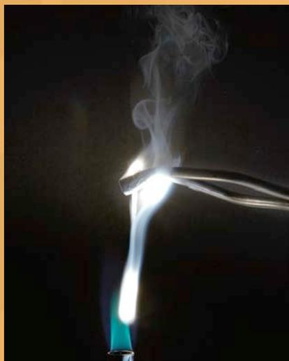
Magnesium burns in air to give magnesium oxide
