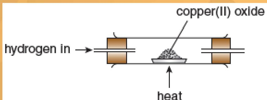
When hydrogen is passed over heated copper(II) oxide, the oxide is reduced to copper
