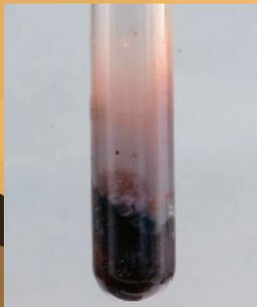
**Steamy fumes of hydrogen iodide and a black solid of iodine are formed when concentrated sulphuric acid reacts with sodium iodide**
