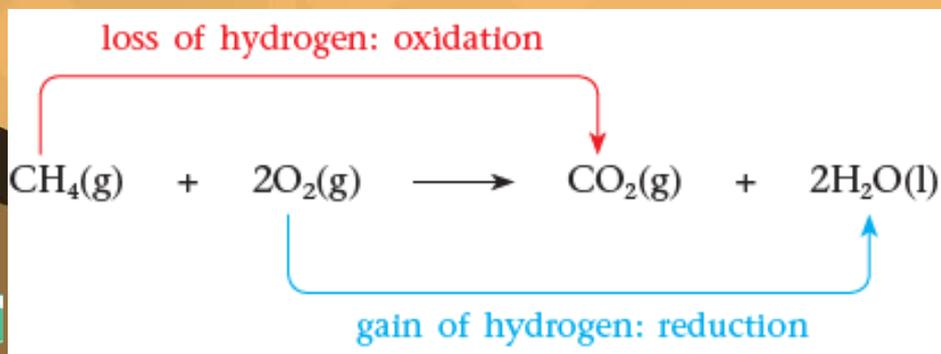
The redox reaction that occurs when methane burns completely in oxygen
