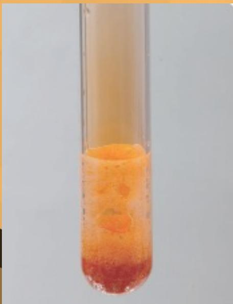
**Steamy fumes of hydrogen bromide and brown fumes of bromine are produced when concentrated sulphuric acid reacts with sodium bromide**
