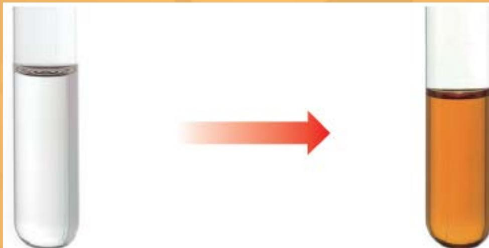
$\text{I}^{-}(\text{aq})$  ions (left) are oxidised to  $\text{I}_2(\text{aq})$  (right) during a redox reaction
