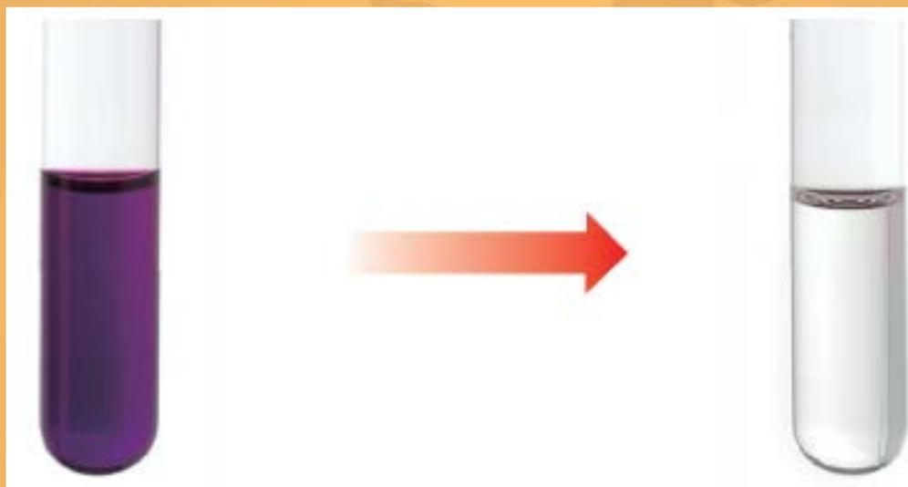
**$\text{MnO}_4^-(\text{aq})$  ions (left) are reduced to  $\text{Mn}^{2+}(\text{aq})$  ions (right) during a redox reaction**
