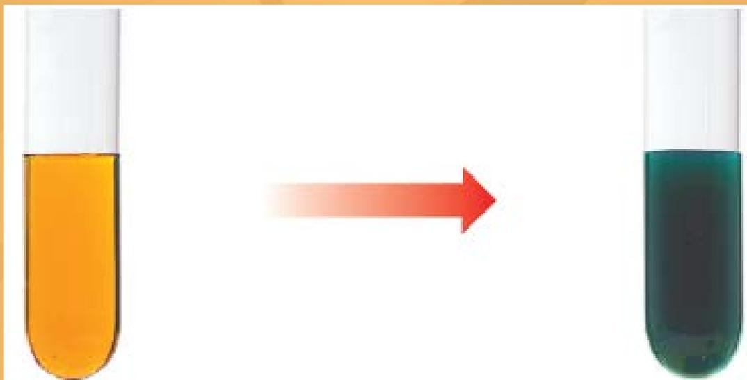
$\text{Cr}_2\text{O}_7^{2-}(\text{aq})$  ions (left) are reduced to  $\text{Cr}^{3+}(\text{aq})$  ions (right) during a redox reaction
