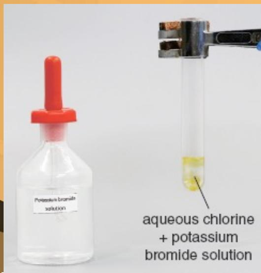
**Aqueous chlorine reacts with potassium bromide solution to form bromine**
