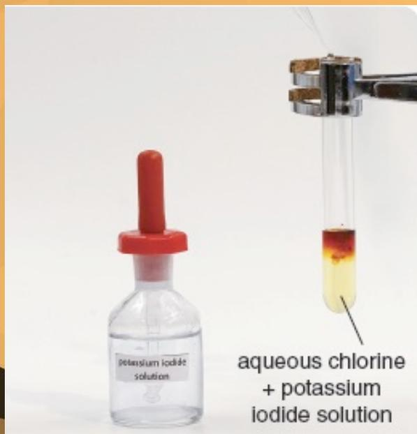
**Aqueous chlorine reacts with potassium iodide solution to form iodine**
