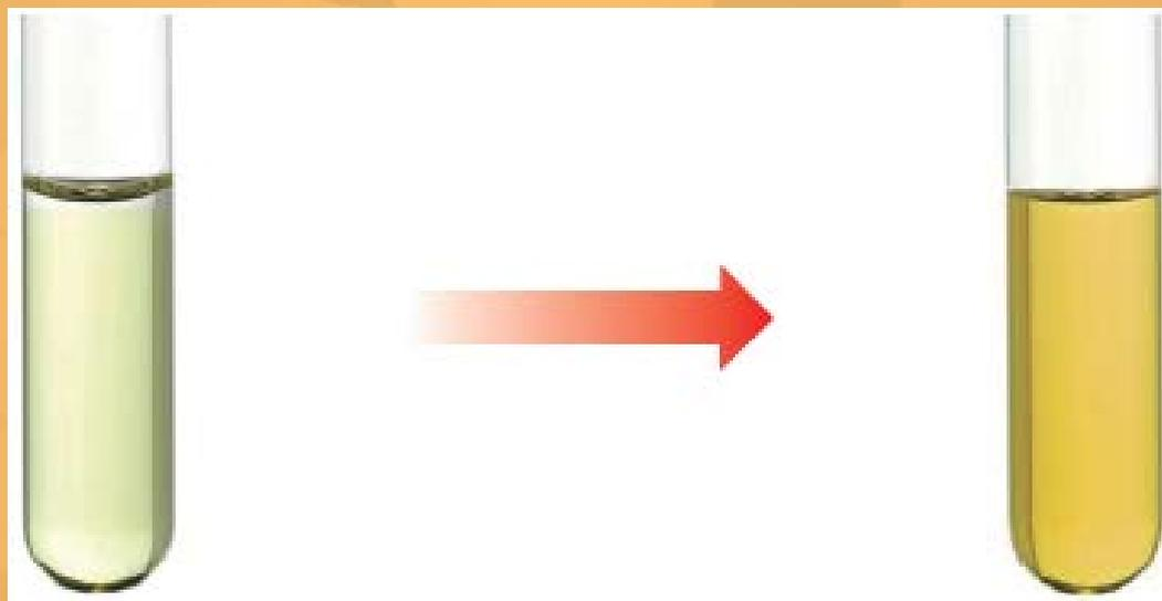
**Fe<sup>2+</sup>(aq) ions (left) are oxidised to Fe<sup>3+</sup>(aq) ions (right) during a redox reaction**
