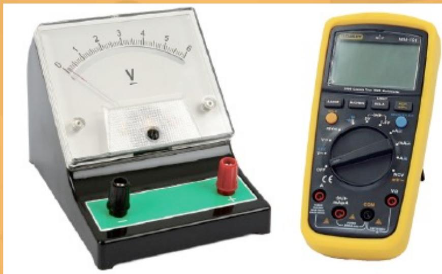
A voltmeter (left) and a digital multimeter (right)
