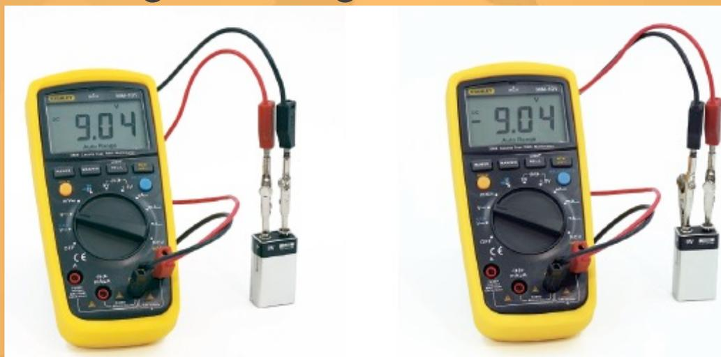
**Reversing the electrodes of a chemical cell with respect to the multimeter changes the sign on the measured voltage**
