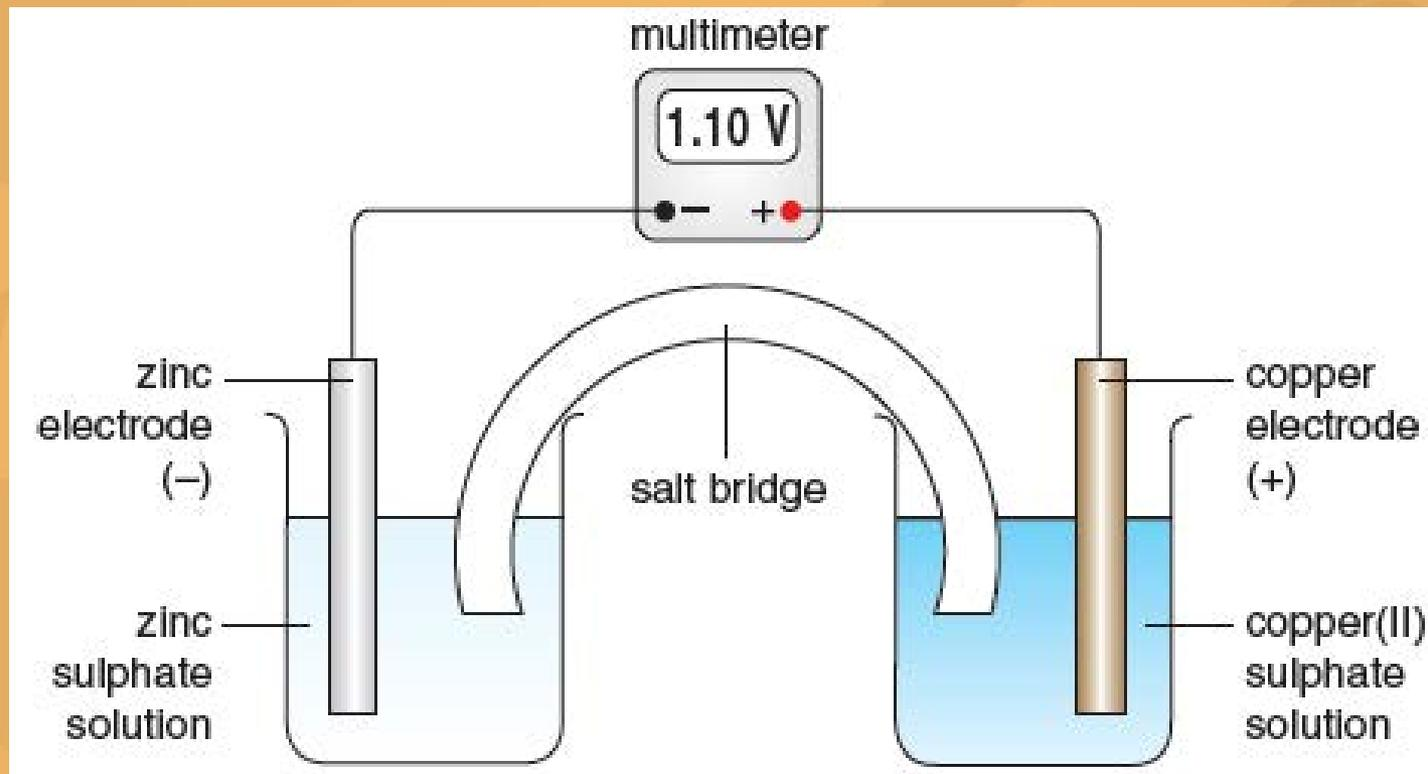
**Building a chemical cell from two half cells**
