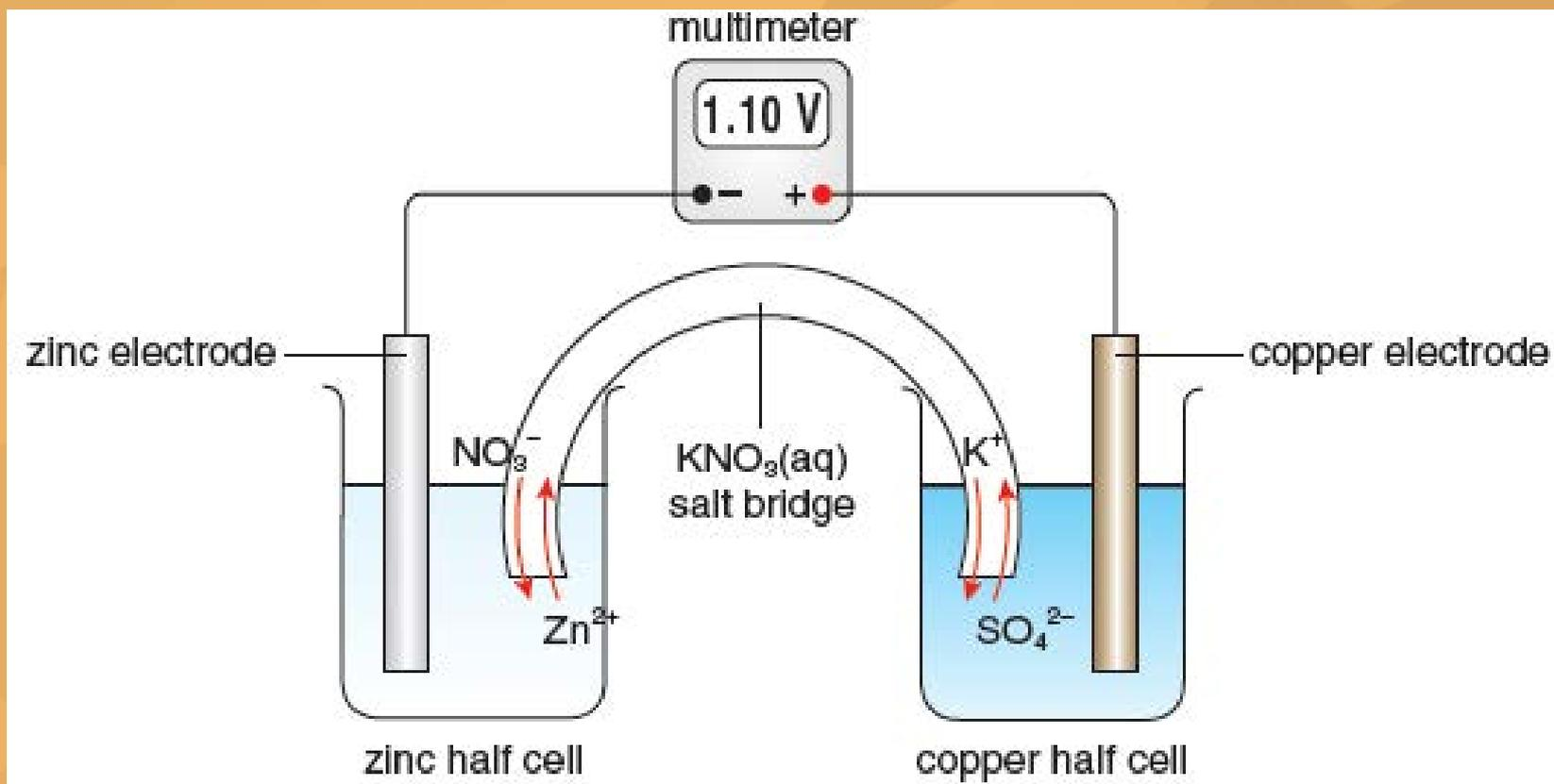
Ions flow into and out of the salt bridge to prevent any build-up of charges in the half cells
