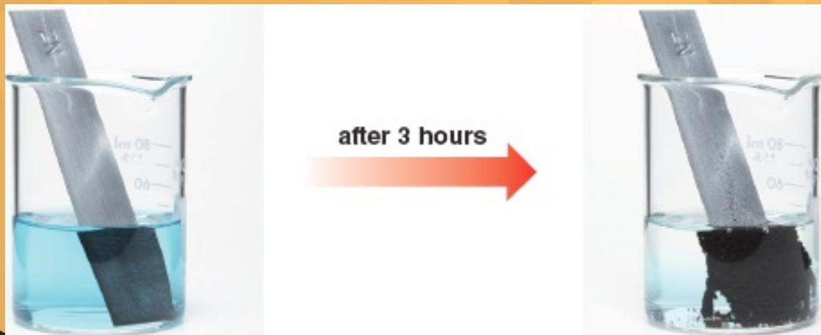
The reaction between zinc and copper(II) sulphate solution
