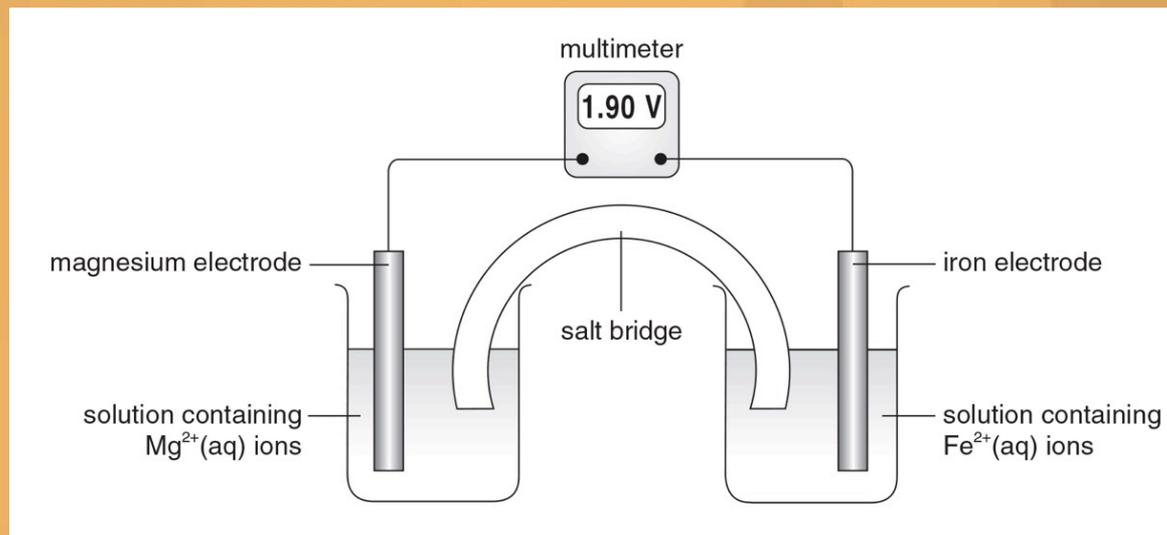
It is found that the concentration of magnesium ions increases as the cell discharges.
