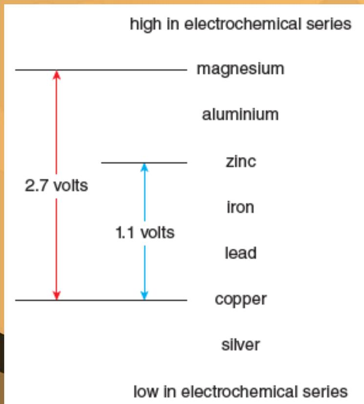
**The further apart between two metals in the electrochemical series, the higher the voltage of a chemical cell**
