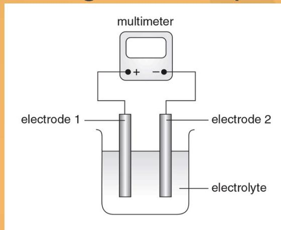
Electrode 1 and electrode 2 are made from two different metals. The voltage of the chemical cell is recorded. The table below shows the results obtained.
