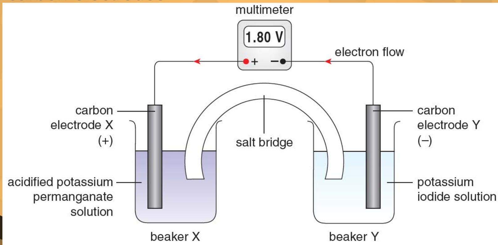
**A chemical cell with carbon electrodes**
