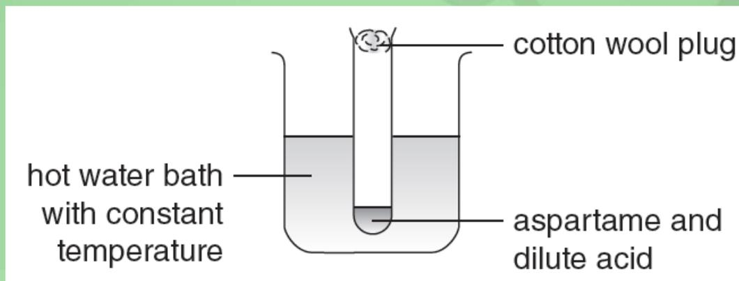
What improvement could be made to the apparatus to reduce the loss of methanol by evaporation?
