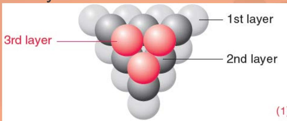
Draw a third layer of atoms on the diagram to show the 'ABCABC' stacking pattern.
