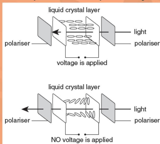
Explain why the pixel appears dark when a voltage is applied to the liquid crystal layer.
