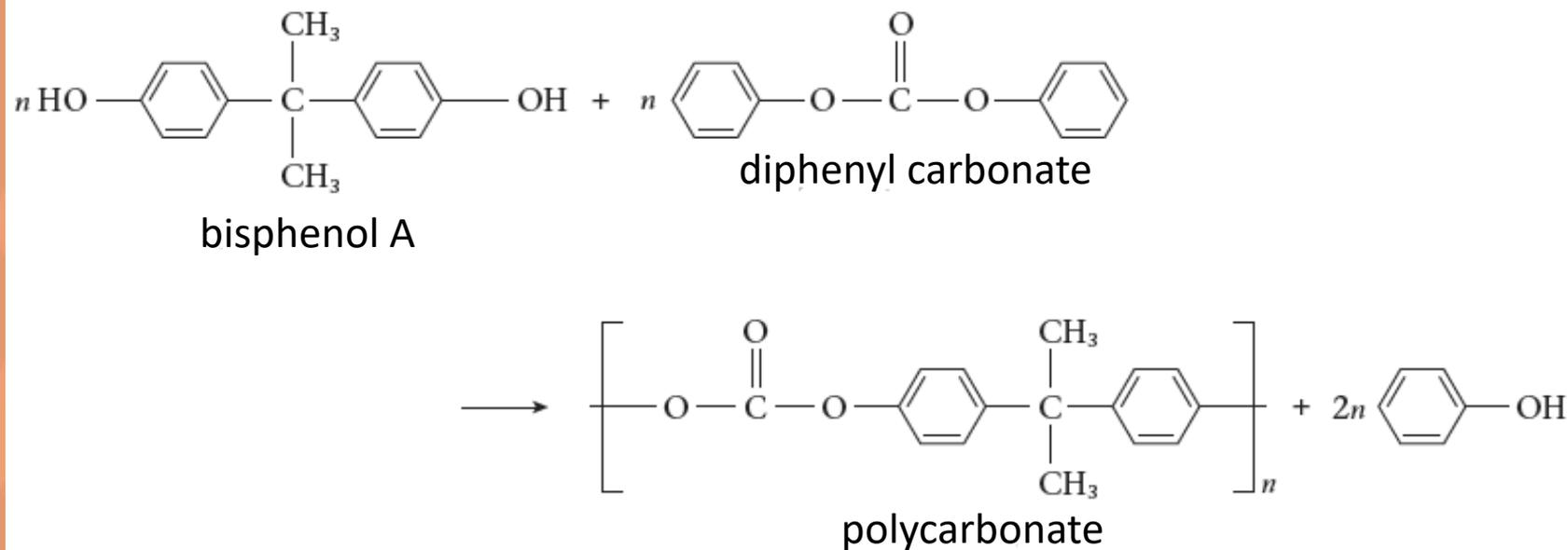
This non-phosgene process does not use the highly toxic phosgene. It also avoids the use of chlorinated organic solvent and the production of sodium chloride. This process has gradually replaced the phosgene process.
