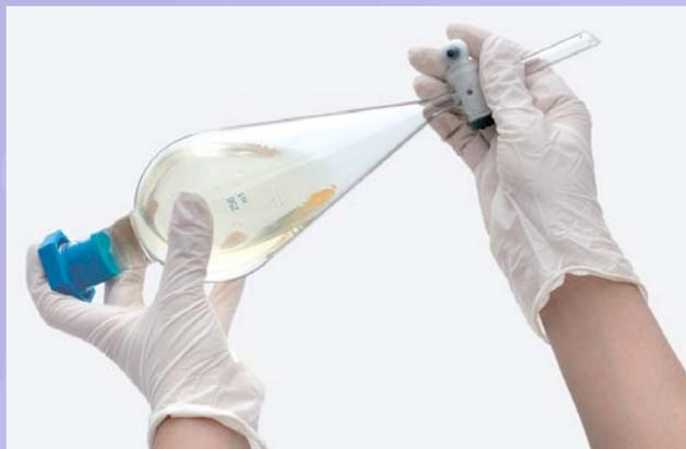
**Hold the stopper and the tap firmly when shaking**
