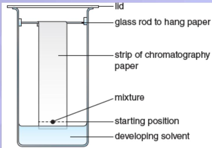
**A chromatography tank (the sample spot on the paper must be above the level of the solvent)**
