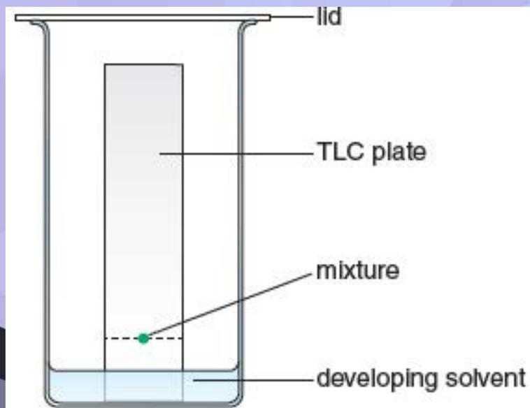
The apparatus used for thin layer chromatography (TLC)
