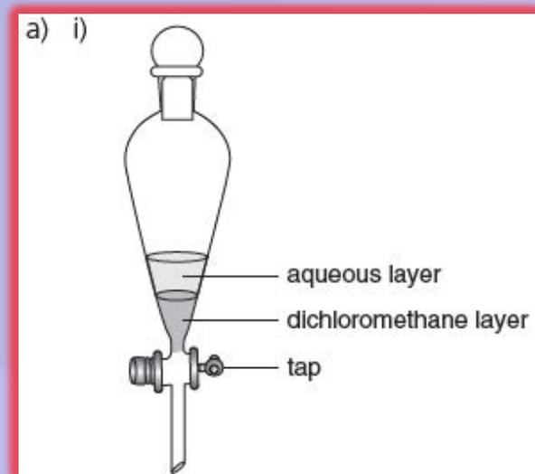
Open the tap of the separating funnel regularly to release the pressure built up inside the funnel.
