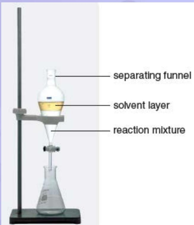
**During the extraction, add a solvent to the reaction mixture, giving two layers of liquids**
