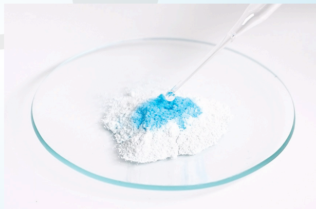
Anhydrous copper(II) sulphate changes from white to blue when water is added to it
