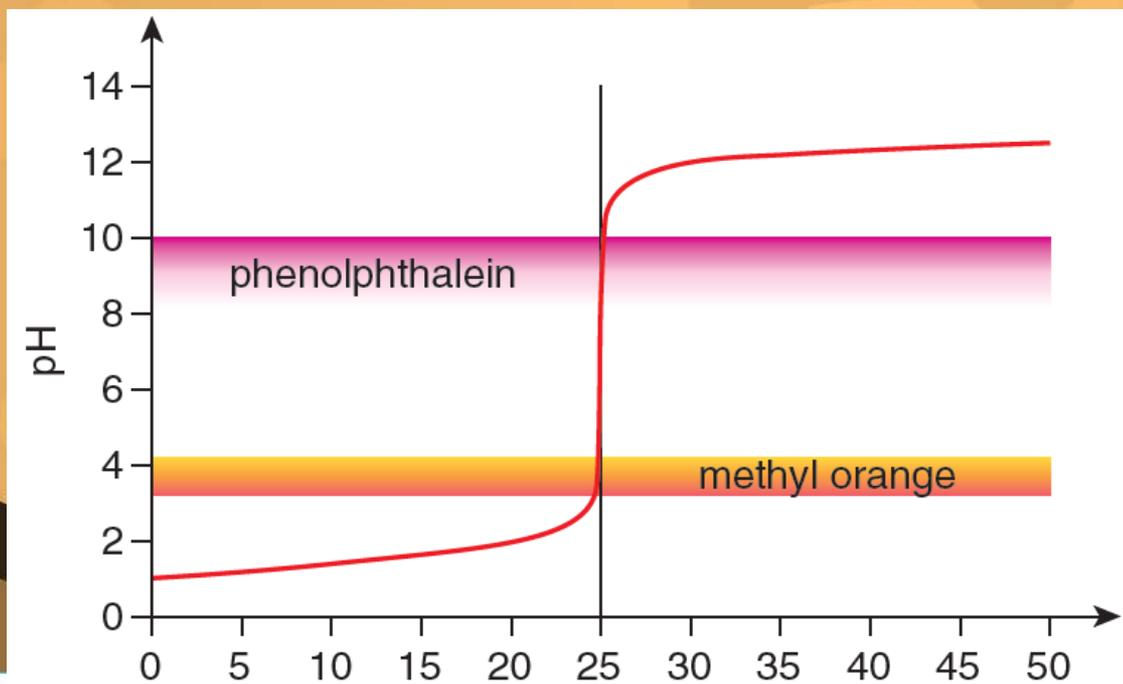
Titration curve of a strong acid-strong alkali titration, adding  $0.1 \text{ mol dm}^{-3} \text{ NaOH(aq)}$  to  $25.00 \text{ cm}^3$  of  $0.1 \text{ mol dm}^{-3} \text{ HCl(aq)}$
