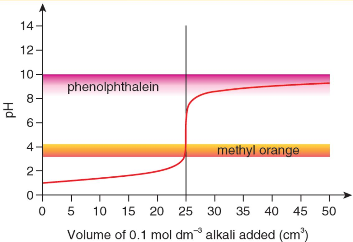
Titration curve of a strong acid-weak alkali titration, adding 0.1 mol dm<sup>-3</sup> NH<sub>3</sub>(aq) to 25.00 cm<sup>3</sup> of 0.1 mol dm<sup>-3</sup> HCl(aq)
