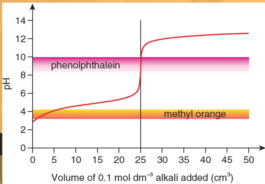
**Titration curve of a weak acid-strong alkali titration, adding 0.1 mol dm<sup>-3</sup> NaOH(aq) to 25.00 cm<sup>3</sup> of 0.1 mol dm<sup>-3</sup> CH<sub>3</sub>COOH(aq)**
