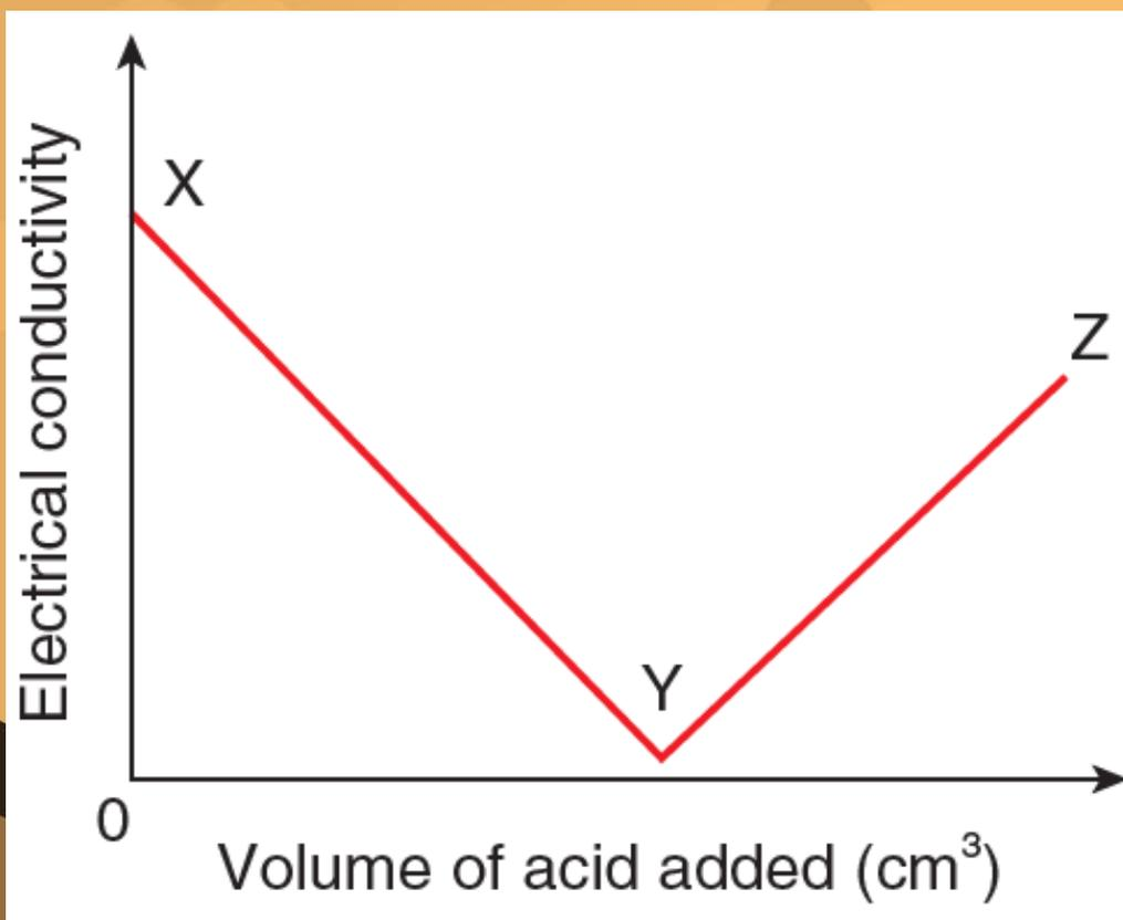
The change in electrical conductivity of the reaction mixture when dilute sulphuric acid is added gradually to barium hydroxide solution
