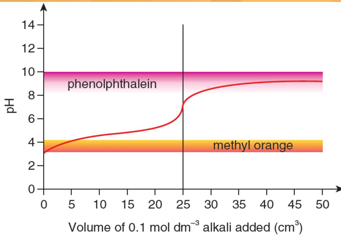
Titration curve of a weak acid-weak alkali titration, adding  $0.1 \text{ mol dm}^{-3} \text{ NH}_3(\text{aq})$  to  $25.00 \text{ cm}^3$  of  $0.1 \text{ mol dm}^{-3} \text{ CH}_3\text{COOH}(\text{aq})$
