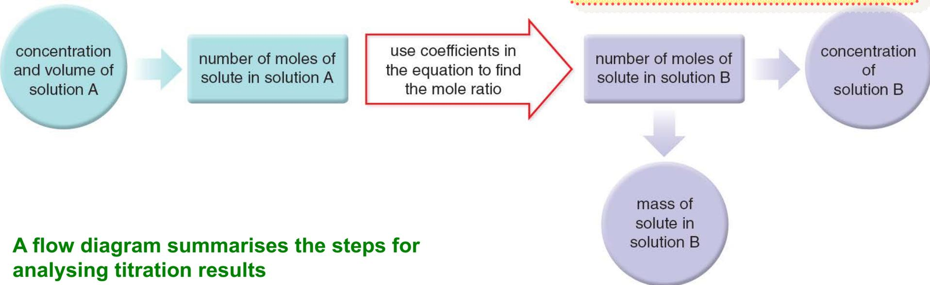
**A flow diagram summarises the steps for analysing titration results**
