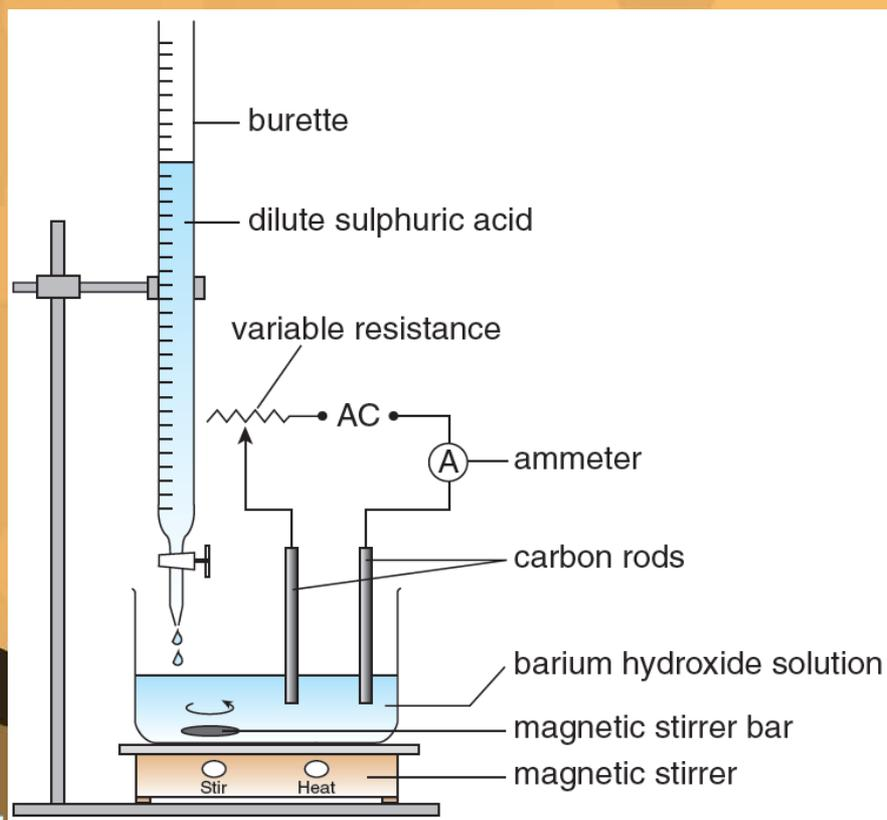
**Experimental set-up for monitoring the electrical conductivity of the reaction mixture when dilute sulphuric acid is added gradually to barium hydroxide solution**
