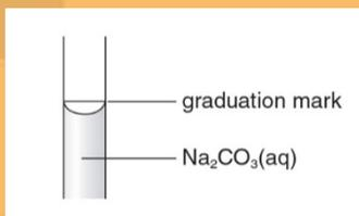
*Step 3* Standard Na<sub>2</sub>CO<sub>3</sub>(aq) in the pipette was transferred to the conical flask. To ensure that all the solution was transferred, the student blew through the pipette.
