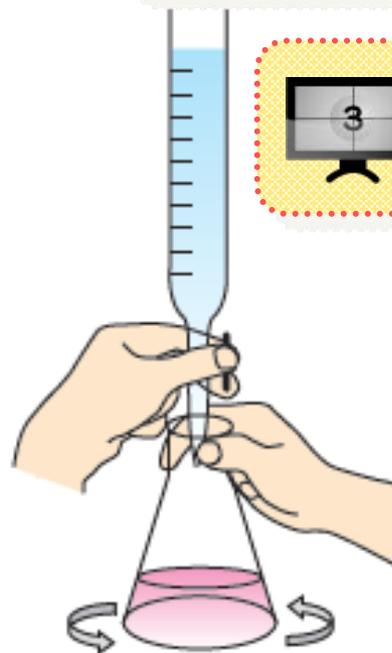
**3** Add a few drops of phenolphthalein to the conical flask. Put the flask on a white tile under the burette.
