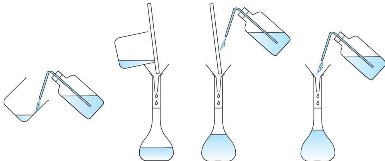
5 Transfer the solution to a  $250.0 \text{ cm}^3$  volumetric flask with the aid of a filter funnel.
