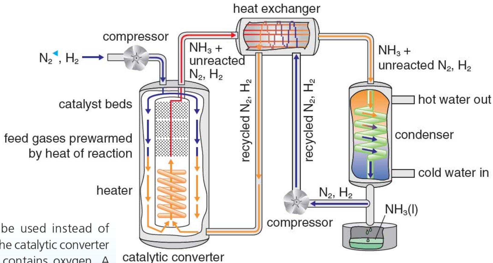
Air cannot be used instead of nitrogen in the catalytic converter because air contains oxygen. A mixture of oxygen and hydrogen is explosive.
