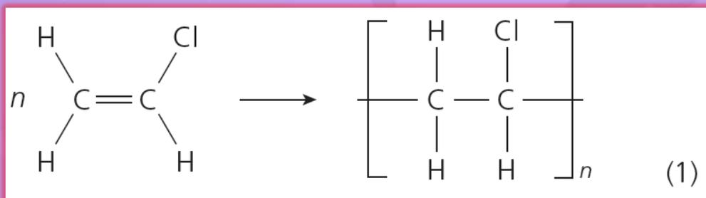
It is used in making pipes / used in wire and cable insulation. (1)
