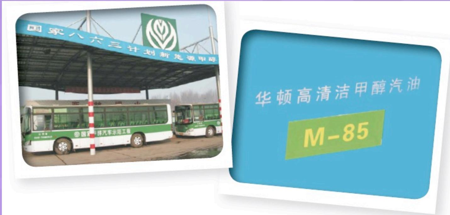
**M-85 is a blend of 85% methanol and 15% petrol; this can be used in vehicles with modified engines**
