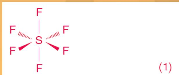
The six bond pairs in the outermost shell of the central sulphur atom stay as far part as possible to minimise repulsion and an octahedral arrangement results. (1)
