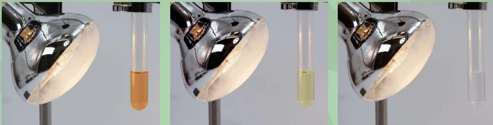
The effect of light on a mixture of bromine and hexane after 0, 10 and 16 seconds
