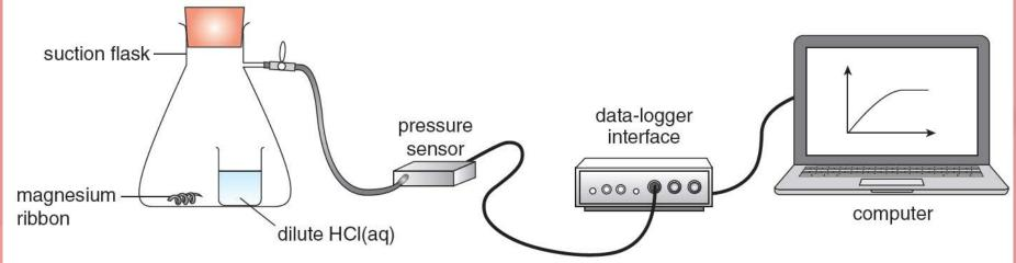
The variation of the pressure inside the closed container with time
