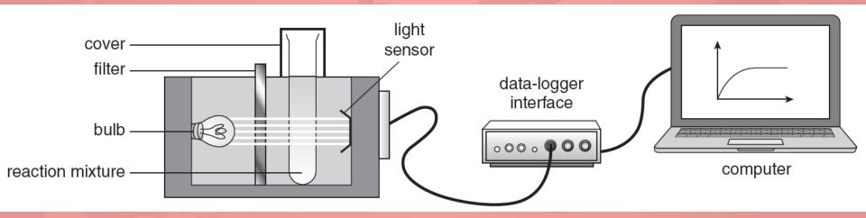
Continous readings / graph of light transmittance of reaction mixture against time plotted automatically. (1)
