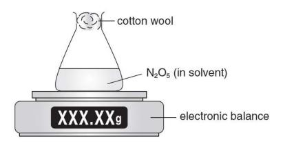
Measurements: mass loss and time
