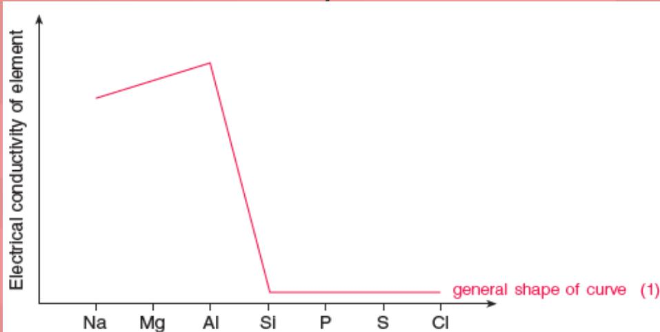
Sodium, magnesium and aluminium have giant metallic structures. They have high electrical conductivities due to the presence of delocalised electrons in the structures. (1)
