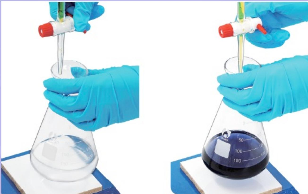
Standard aqueous solution of iodine is run from the burette into the vitamin C solution (left); the first appearance of a persistent dark blue colour indicates the titration end point (right)
