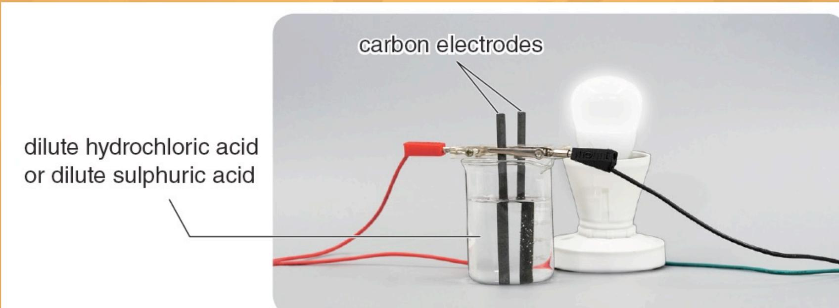
**Experimental set-up to test the electrical conductivity of a dilute acid**
