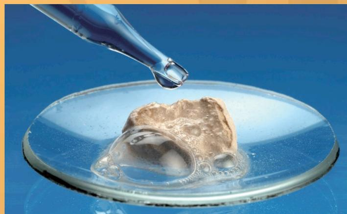
**A rock containing carbonate gives carbon dioxide gas with dilute hydrochloric acid**
