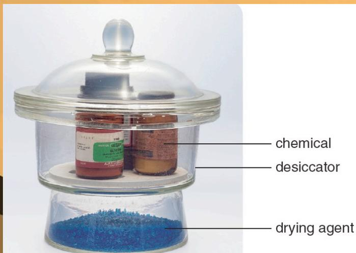
Using a drying agent in a desiccator for maintaining a dry environment for the chemicals
