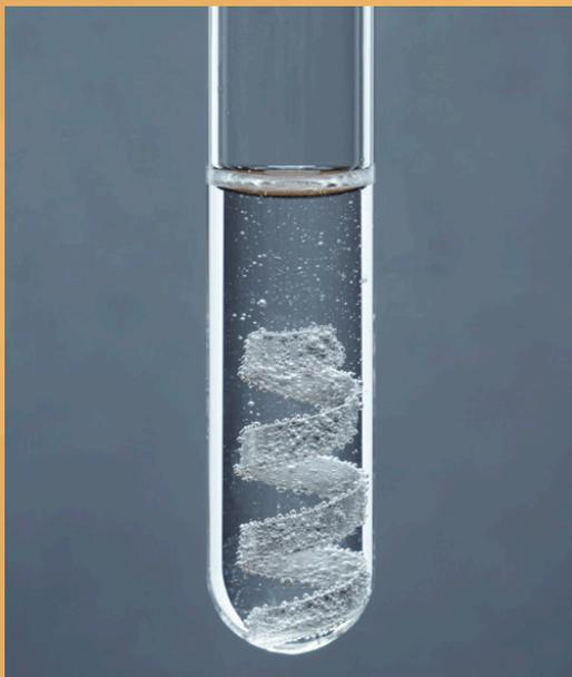
**Magnesium ribbon reacting with dilute hydrochloric acid — giving off hydrogen**
