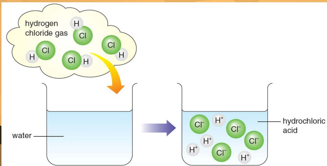
The HCl molecules dissociate in water to form ions
