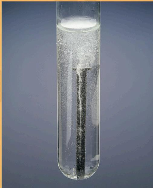
**Iron reacting with dilute sulphuric acid — giving off hydrogen**
