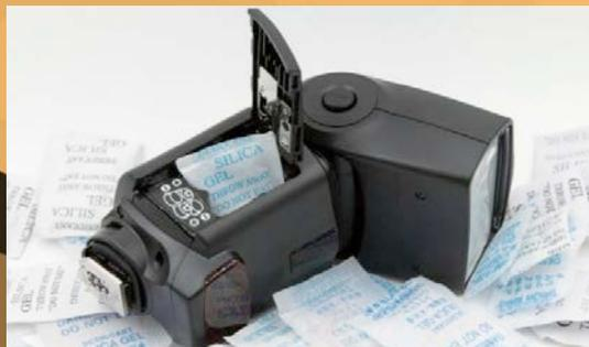
**Silica gel is used as a drying agent to keep the camera flashlight dry**
