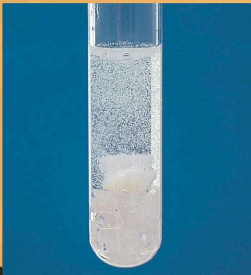
**Calcium carbonate reacts with dilute hydrochloric acid to give carbon dioxide gas. Effervescence occurs as a result**
