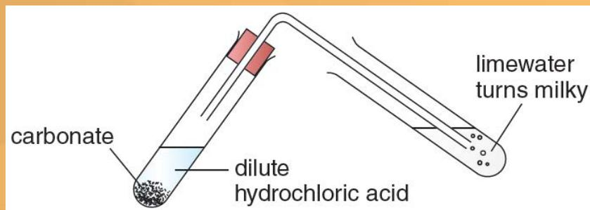
**A carbonate gives carbon dioxide with dilute hydrochloric acid**
