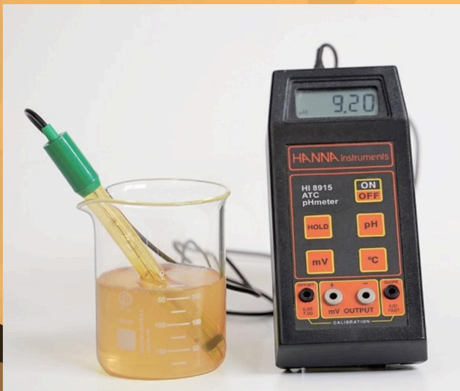
A pH meter with an electrode in an alkaline solution
